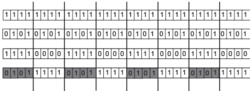
The shaded boxes show the bits that changed in value_b
